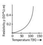
The variation of resistivity of copper with temperature is as shown in figure.
