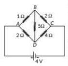
$$I_1R_1 + I_2G - (I - I_1)R_3 = 0$$
